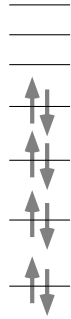
Figure 2. A schematic diagram of the ground state of a non-interacting many-electron system. The lowest N_e/2 single-electron energy levels are ‘filled’ by both up-spin and down-spin electrons. The state naturally exhibits a type of paramagnetism known as Pauli paramagnetism.
